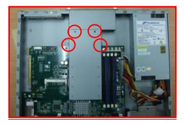
Step 8: Lock the cables in position and done the CPU installation
