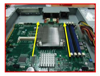
Step 7: Fasten the four screws to lock the air duct
