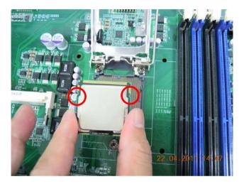
Step 5: Close the CPU bracket and lock the pole to the position
