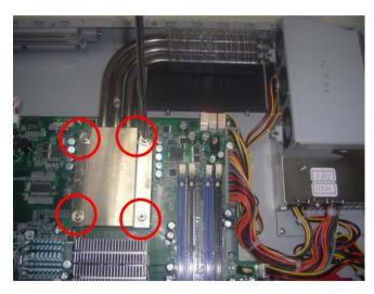
Step 11: Put the fan module back to the original place, and fasten these two screws of the fan module
