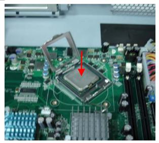
Step 5: Lock the CPU Socket
