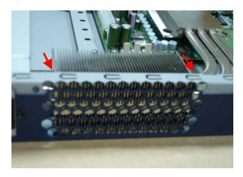
Step 10: Fasten the four screws of the heatpipe
