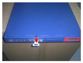
Step 3: Insert the LAN Module and fasten the screws
