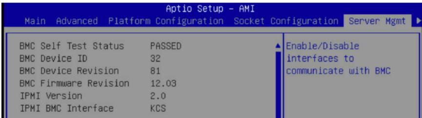
**Step 4:** To configure the BMC IP address, select **Server Mgmt > BMC network configuration**. The user can set the BMC IP source to **Static**, **DynamicBmcDhcp**, or **DynamicBmcNonDhcp**, then reset the system. For the below user guide example, we have selected **DynamicBmcDhcp**. After reset, BMC will get the IP from the DHCP server.
