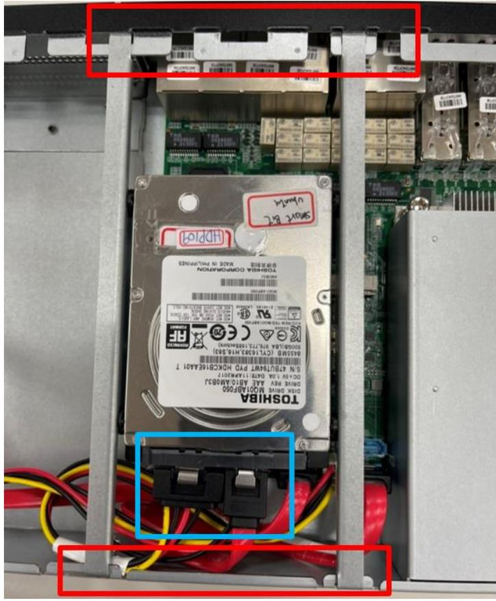
**Step 6:** Connect the SATA cable and power cable into the Hard Disk and put hard drive bracket on the chassis.
