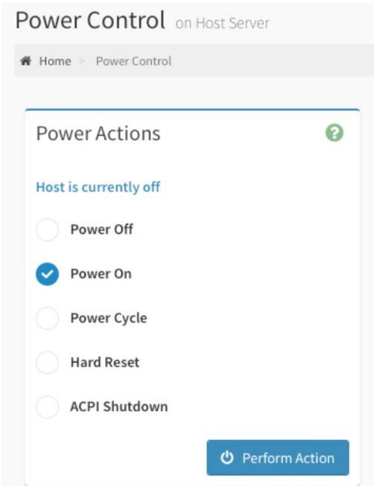
**Step 3:** When the host status is on, the user can select actions including **Power Off**, **Power Cycle**, **Hard Reset**, and **ACPI Shutdown**. See below for a description of each power action.
