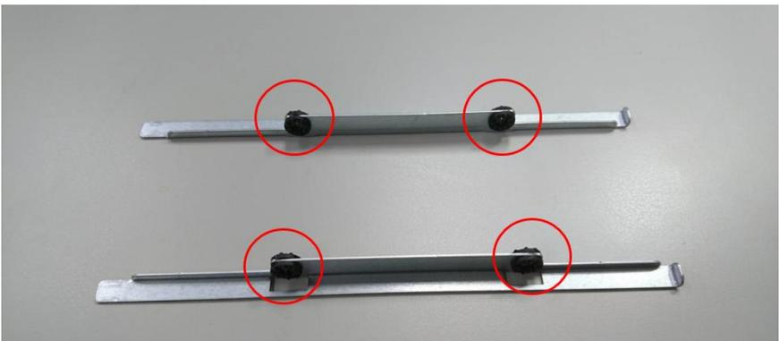
**Step 3:** Lock HDD on the bottom cushions with four screws.
