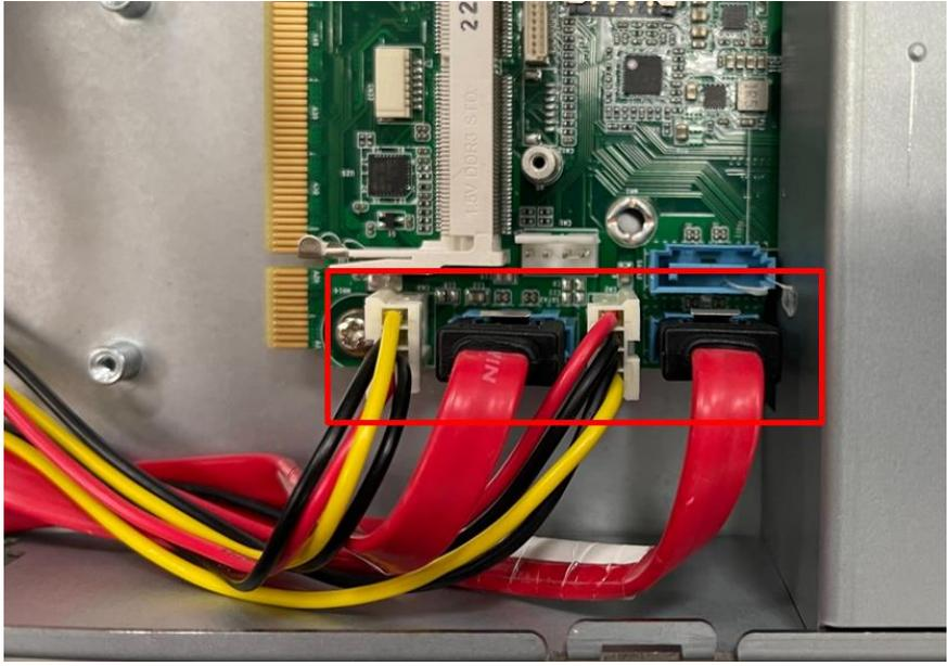
**Step 5:** Connect the SATA cable and power cable into the Hard Disk and put hard drive bracket on the chassis.
