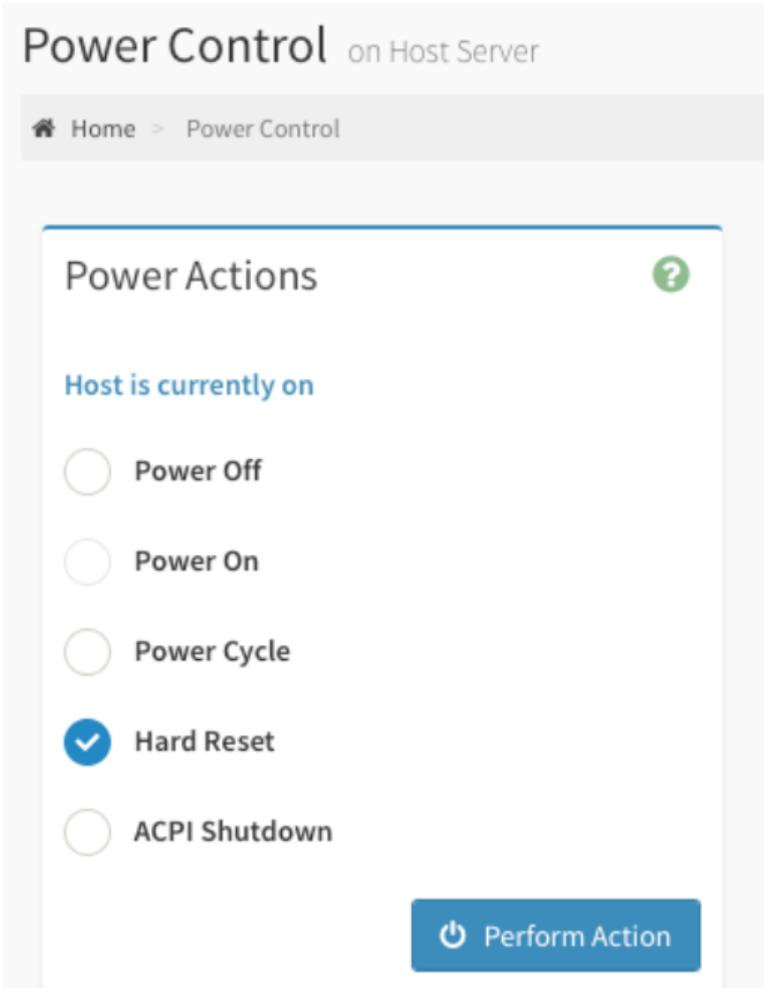
**Step 2:** When the host status is off, the only action that can be selected is **Power On**. Select this and press **Perform Action** to boot the host.
