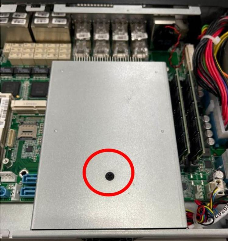
**Step 2:** Cover the Heatsink on the CPU and ensure the direction of the Heatsink does not obstruct the airflow.
