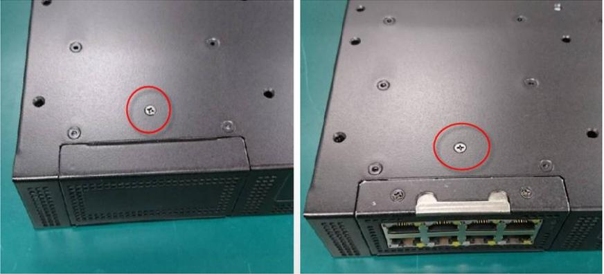
**Step 2:** Remove the null Module cover or existing LAN module.
