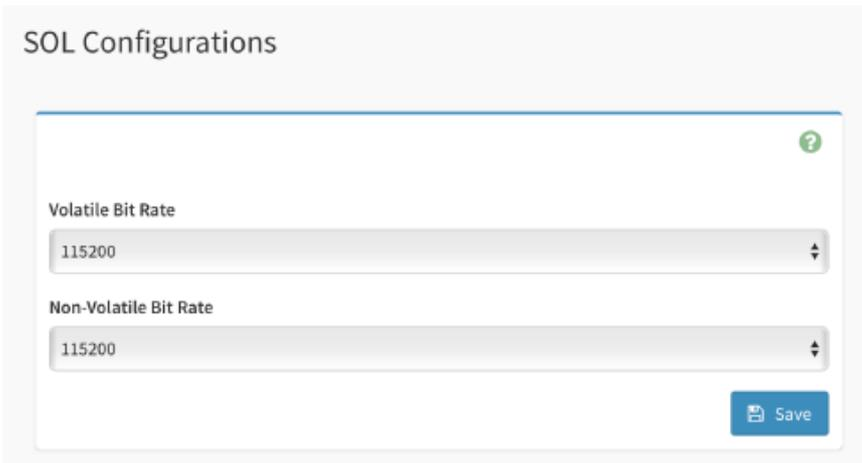
The screenshot displays the 'SOL Configurations' web interface. It features two input fields for bit rates, both set to '115200'. The first field is labeled 'Volatile Bit Rate' and the second is labeled 'Non-Volatile Bit Rate'. A blue 'Save' button is located at the bottom right of the configuration area. A green question mark icon is visible in the top right corner of the configuration box.
