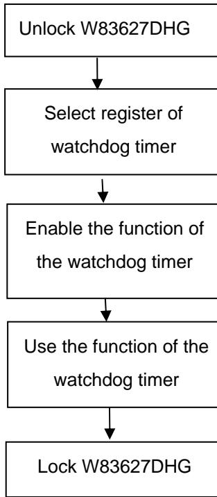
There are three steps to complete the configuration setup:
