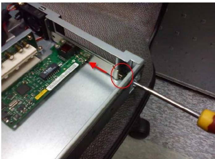
Step 6: Lift down the upper expansion card and push into the slot. Fix the expansion card with screws
