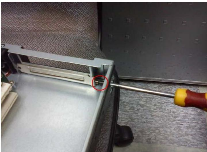
Step 5: Lift down the lower expansion card and push into the slot. Fix the expansion card with screws
