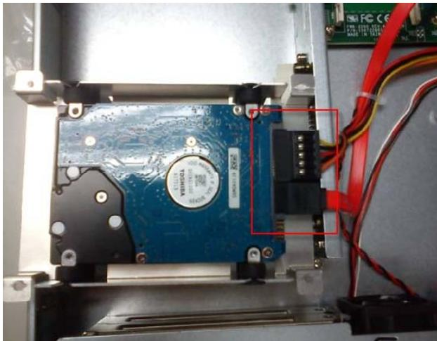
Step 9: Lock HDD bracket on the chassis with four screws
