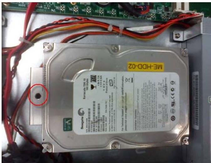
Step 7: Connect the SATA cable and power cable to the HDD
