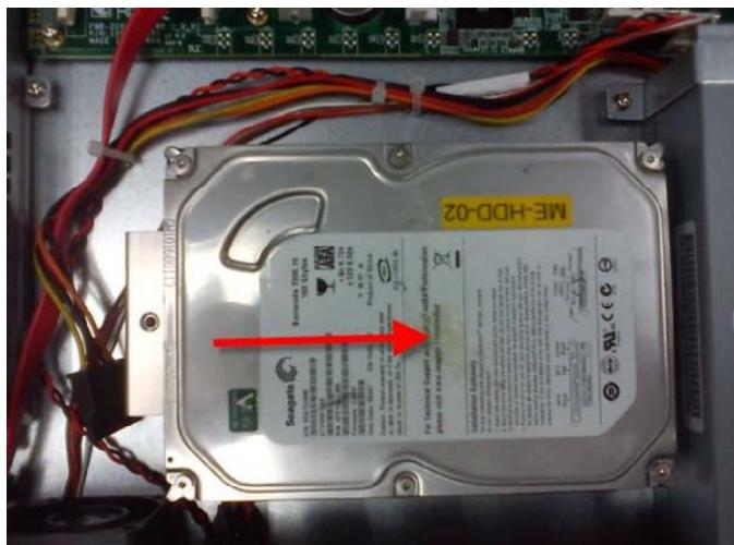
Step 6: Lock the HDD bracket with a screw
