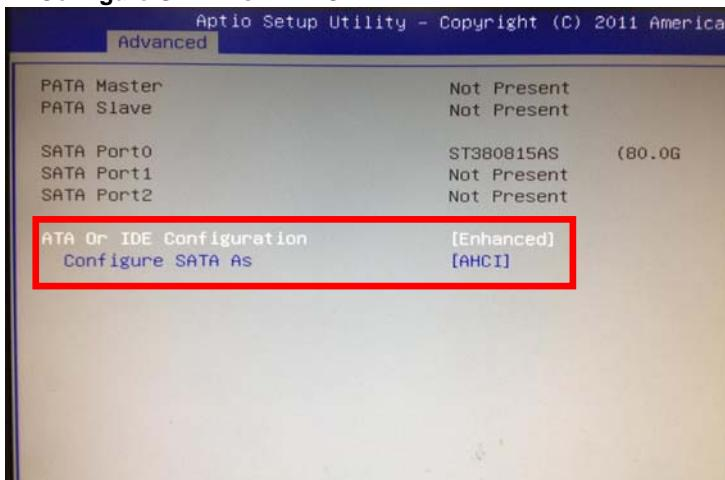
Step 4: The setting procedures “**In BIOS Setup Menu**”
