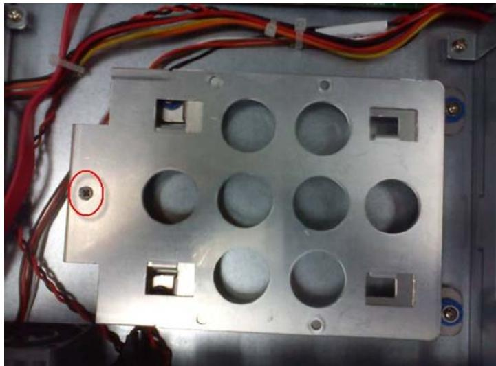
Step 3: Slide the upper HDD bracket and separate the two pieces of HDD brackets
