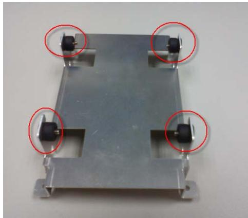
Step 5: put assembled cushions on the bottom HDD bracket
