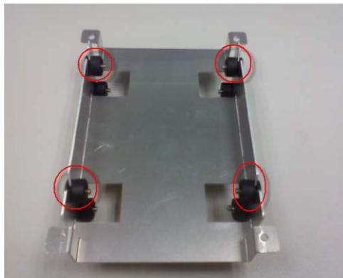
Step 6: Lock HDD on the bottom bracket with four screws
