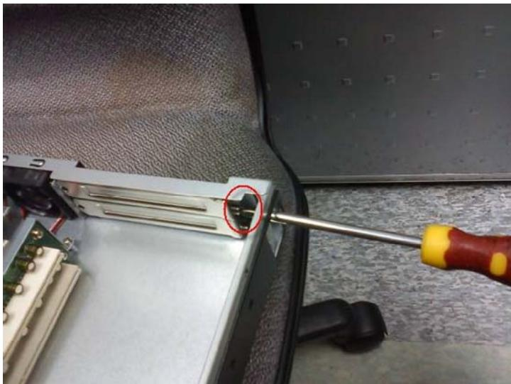
Step 4: Unfasten the screw and lift up the lower I/O bracket
