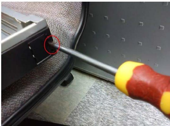
Step 3: Unfasten the screw and lift up the upper I/O bracket
