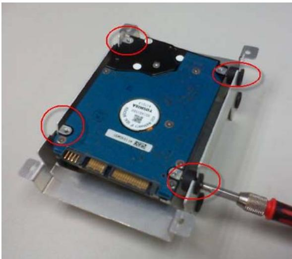
Step 7: Lock the HDD on the upper bracket with four screws
