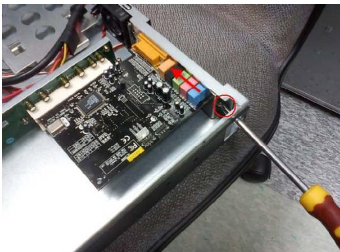
Step 7: Close the cover bracket and fasten the cover with screws
