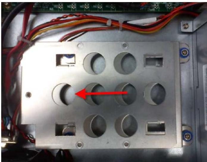
Step 4: Put on the HDD in the drive bay and lock with four screws
