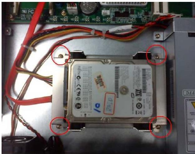
Step 10: Connect the SATA cable and power cable to the Hard Disk
