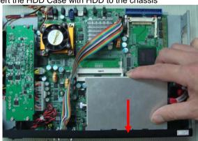
Step 6: Lock the HDD case horizontally
