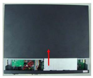
Step 2: Take out the HDD Case from the chassis
