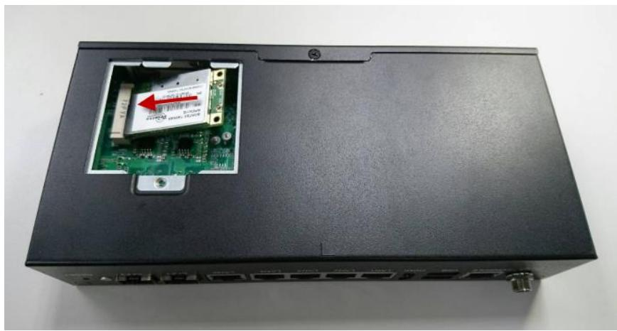
3. Lock down the Mini PCIe card with the screw.
