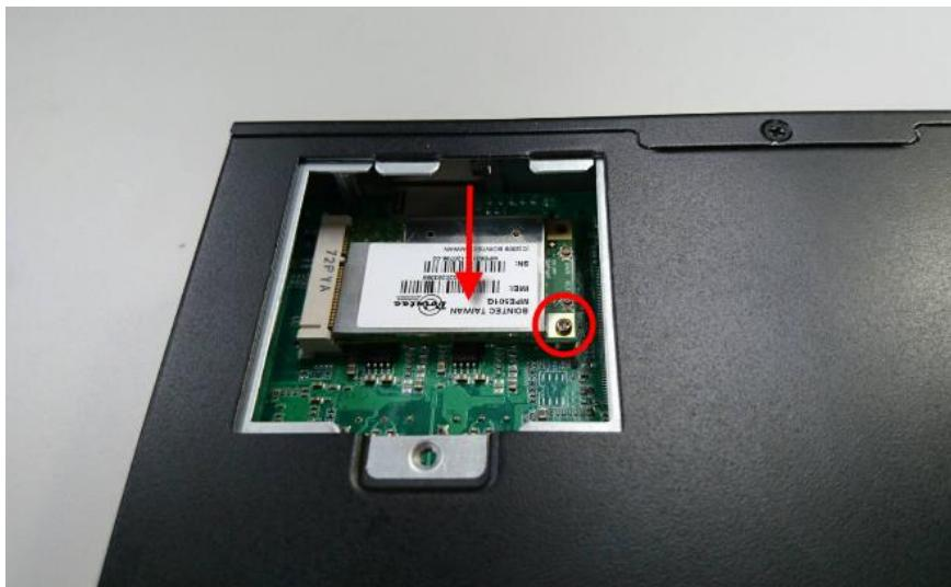
4. Lock down the Mini PCIe card cover with the screw.
