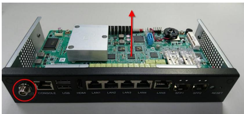
3. Loosen the four screws and remove the mother board.
