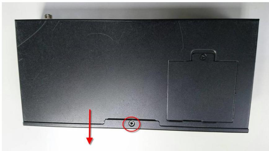
2. Loosen the screw and remove the mother board module.
