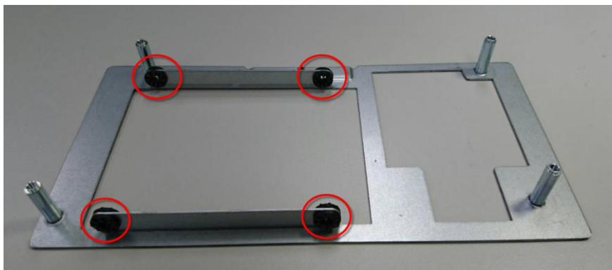
5. Lock the HDD onto the cushions with the four screws
