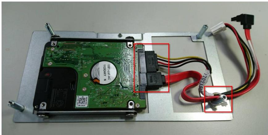
7. Connect the SATA cable and the power cable onto the mother board, and lock in the mother board with the four screws.
