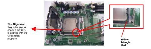
d. Close the upper plate (A), place the load lever back to the original position and tightly wedge the lever into the fastening tab. (B)
