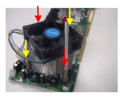
e. Connect the CPU fan cable to the power connector labeled FAN1 on the board.
