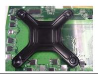
Viewing the board again from the topside make sure the bracket on the solder side has not shifted from its position. Daub thermal compound on the CPU.
