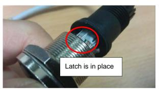
Step 6: Lock and tighten the nut of RJ-45 plug
