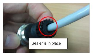
Step 8: Before locking the plastic rear nut tightly, press the cable hardly and make sure all parts of the LAN connector has been connected tightly
