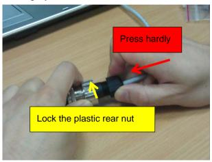
Step 9: Tighten the plastic rear nut again to make sure the cable is securely connected and would not fall off accidentally
