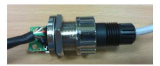
Step 7: Screw on the plastic rear nut a little bit for locking later. Make sure sealer is in place
