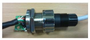
Step 7: Screw on the plastic rear nut a little bit for locking later. Make sure sealer is in place
