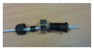
Step 4: Install and crimp a new RJ-45 plug
