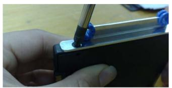
Step 4: Put HDD on the bottom case of FES-6110 and then fasten 4 screws to fix on it.
