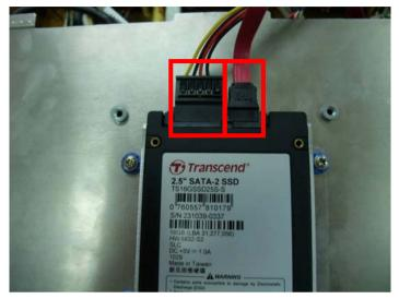
Step 8 : HDD installation finished.
