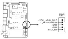
**EPC-CV1** Backlight inverter power connector
