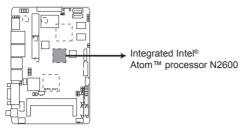
EPC-CV1 Integrated Intel<sup>®</sup> Atom™ processor N2600
