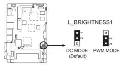
EPC-CV1 LVDS backlight brightness control jumper
