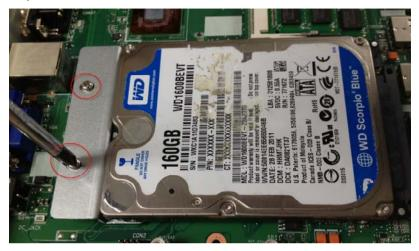
Step 9: Lock the bracket of HDD on the standoff with two screws
