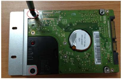
Step 7: Turn the HDD to another side and push it into the slot until connecting firmly
