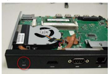
Step 2: Install the connector of antenna
