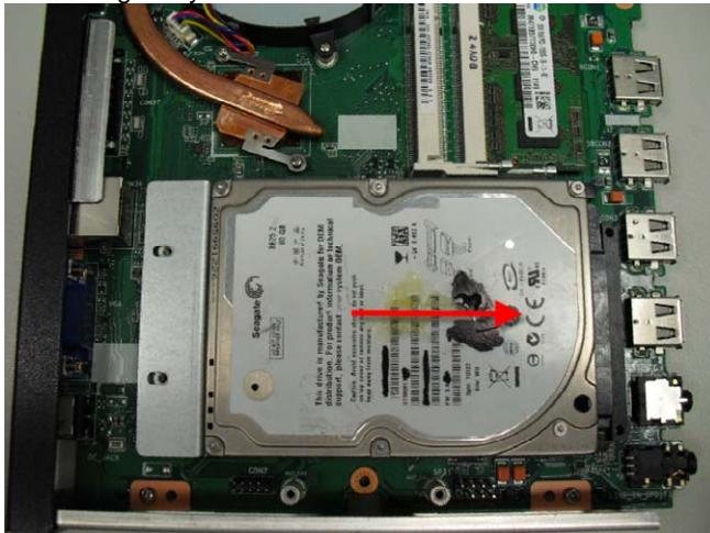
Step 5: Lock the bracket of HDD on the standoff with two screws
