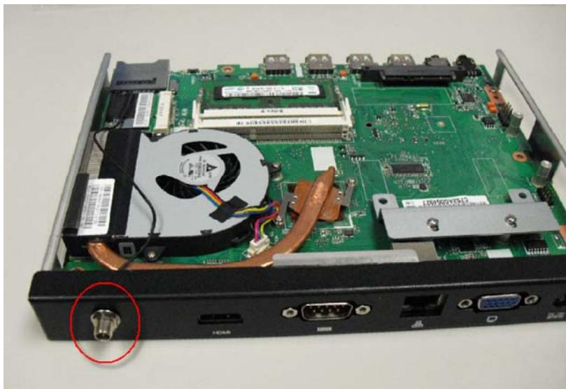
Step 3: Screw the antenna on the connector
