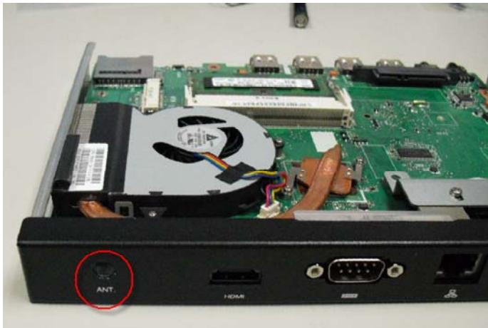
Step 2: Install the connector of antenna
