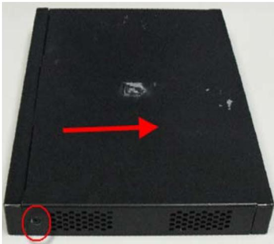
Step 2: Loosen HDD bracket on the standoff with two screws
