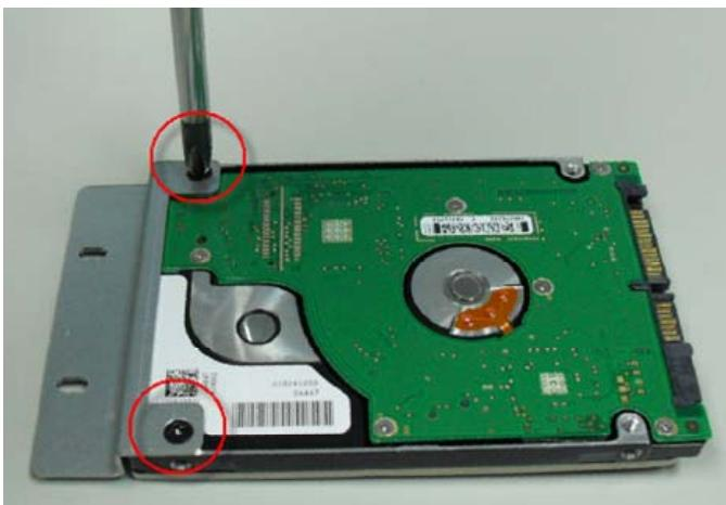
Step 4: Turn the HDD to another side and push it into the slot until connecting firmly
