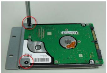
Step 4: Turn the HDD to another side and push it into the slot until connecting firmly
