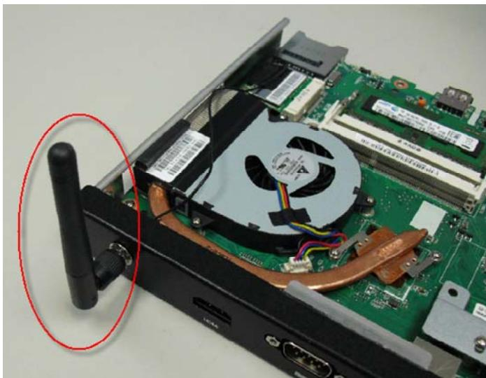
Step 4: Install the Wi-Fi module and fix it by a screw
