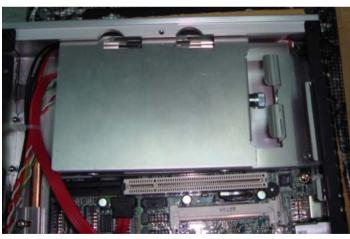
Step 3: Pull out the knob and turn the knob left or right at a 90-degree angle to open the HDD case
