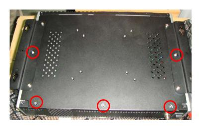
Step 2: Move the HDD case horizontally and take out the HDD case from the DSS-5300
