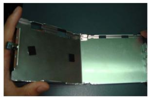
Step 4: Fasten the four screws covered by dampers, which got from the HDD case to the HDD
