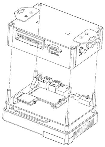
Turn the BOXER-8651AI-Plus system over so the bottom is facing up. Install each bracket using two (2) screws to affix them to the bottom of the chassis, as below.
