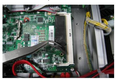
3. Slot in the RAM diagonally, push down to secure.
