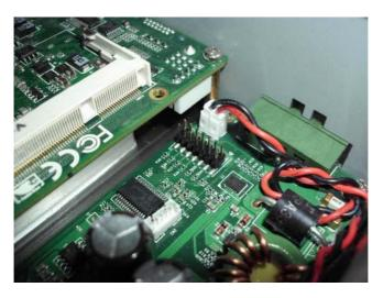
For +24V DC input, a jumper is needed
