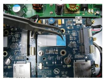
2. Slot the module in diagonally
