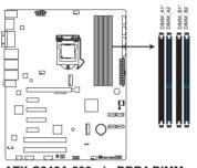
ATX-C246A 288-pin DDR4 DIMM sockets
