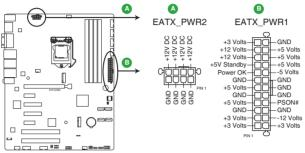
ATX-C246A ATX power connectors
