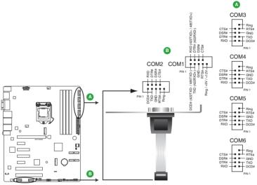
ATX-C246A Serial port (COM) connectors
