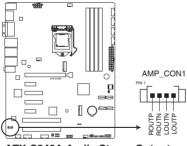
ATX-C246A Audio Stereo Output with Amp connector
