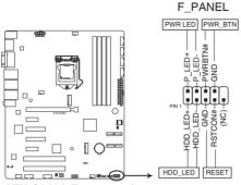
ATX-C246A Front panel connector
