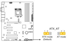
ATX-C246A H/W AT/ATX mode selection
