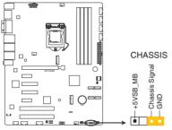
ATX-C246A Chassis intrusion connector
