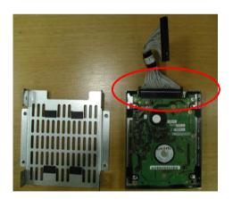
Step 5: Fix the HDD module with screws as follow.
