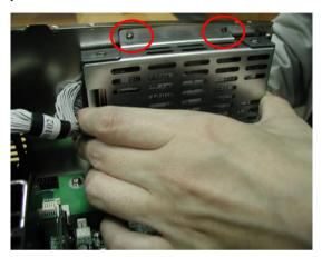
**Step 4:** Insert the IDE cable into HDD and fix the HDD on the bracket with screws.
