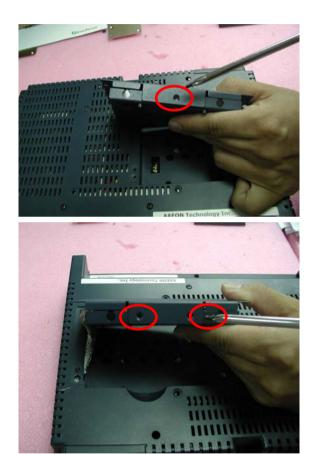
Step 3: Place the HDD with the iron bracket into the concave and fix the HDD with the screws.
