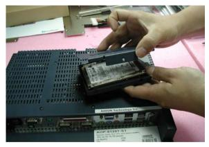
Step 2: Fix two iron brackets with the screws.
