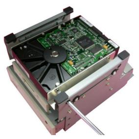
6. Screw the disk drive module to steel chassis and connect the HDD, FDD and CD-ROM cable.
