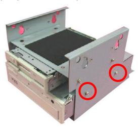
5. Screw 3.5" HDD in bracket.
