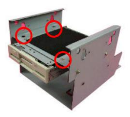
4. Slide the CD-ROM and tighten it. These are four screws separately on each side of metal plate.
