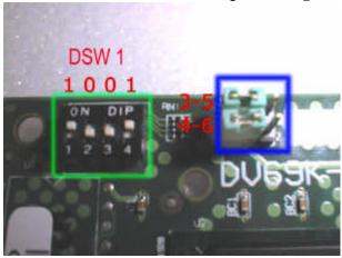
12.1" LCD Panel Jumper setting on DV69K
