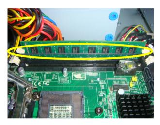
Step 2: Put a rubber band around the RAM to secure it in the slot
