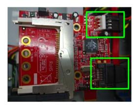
Step 2: Secure the CompactFlash™ card with screws
