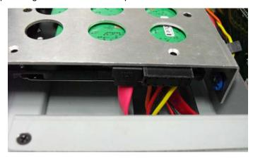
Step 8: Finish the installation. Close and screw the case of the AIS-Q572, and fasten the four screws on the left and right side of the AIS-Q572
