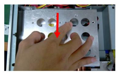
Step 4: Put the HDD to the HDD case and close the upper bracket of the HDD case. And then fasten the four screws on the HDD bracket
