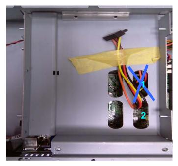
Step 3: After you pull the SATA cable through bracket hole #2, fasten the four screws of the bracket.
