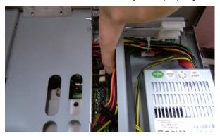
Step 2: The SATA cable will be pulled through bracket hole #2 to avoid damaging the RAM, since the RAM lies directly under bracket hole #1.
