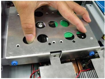
Step 6: Fasten the two screws on the HDD bracket
