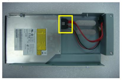
Step 4: Connect the SATA cable onto the main board
