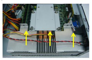
Step 3: Insert screws to secure the heat sink
