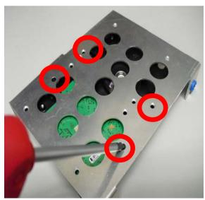
Step 5: Make sure the dampers are inserted to the right place
