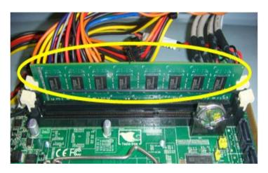
Step 2: Put a rubber band around RAM to secure it in the slot
