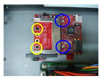
Step 2: Connect the SATA Cable and the Power cable
