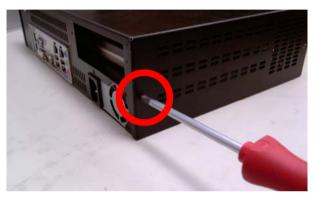
Step 2: Unfasten the two screws on the two sides of the HDD bracket
