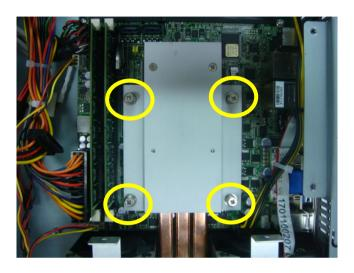
Step 4: Secure bracket and fan with the screws
