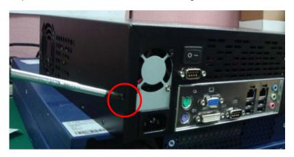
Step 2: Unfasten the screw of the HDD bracket and pull out the bracket
