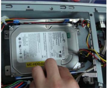
Step 6: Fasten the two screws to lock the HDD bracket
