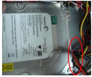
Step 8: Close the upper HDD bracket to the HDD and fasten the screws to lock the HDD kit
