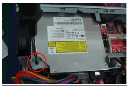
Step 9: Close and screw the case of the AIS-Q454 to finish the installation
