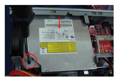
Step 3: Get the HDD ready and place the HDD to the HDD bracket
