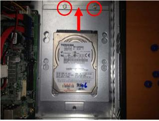
Step 5: Fasten the screw to finish installing the HDD
