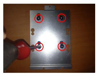
Step 4: Put the HDD and bracket back to the chassis by sliding the HDD bracket and lock to the position.
