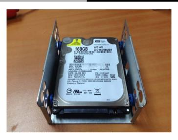
Step 5: Make sure that the fillisters of the 3-layer HDD bracket has been latched to I-shape nails (blue circles)
