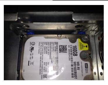
Step 6: Fasten the screw to lock the HDD bracket with the Chassis and you've done installing the three HDD
