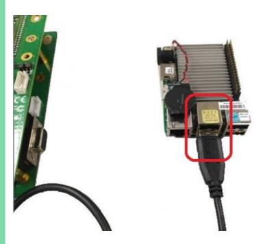
**Step 4:** Plug the HDMI cable \* from your monitor \* in to the HDMI connector on the AAEON computing board.
