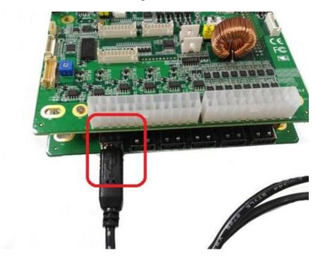
**Step 3:** Plug the type A end of the included USB cable in to one of the USB type A connectors (any USB connector is fine) on the AAEON computing board.
