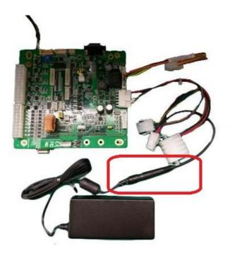
**Step 12:** Plug the AC power cord in to the 24V DC power supply's receptacle. Now plug the 24V DC power supply's AC cord plug in to an 110V AC outlet.
