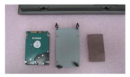
Step 3: Stick the Thermal Pad onto the Hard Disk Drive and fasten the Hard Disk Drive onto the bracket
