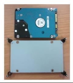
Step 5: Fasten the four screws to fix the HDD with the HDD bracket
