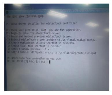
Select the "1" COM interface (Select the COM interface and input command: /dev/ttyS0 (COM1), and press the "Enter" key of the keyboard to start the installation)
