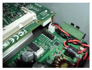
For +24V DC input, there are jumpers on the pin header of the power
