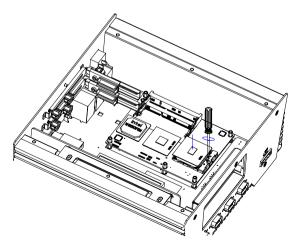
Step 5: Put the thermal pad (1998666628) on the diode of CPU
