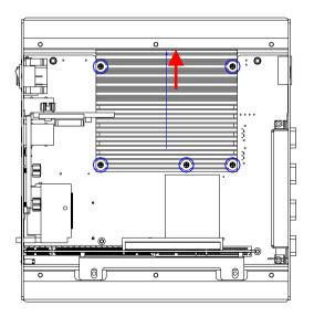
Step 7: Fasten the six screws on the back of the AEC-6940
