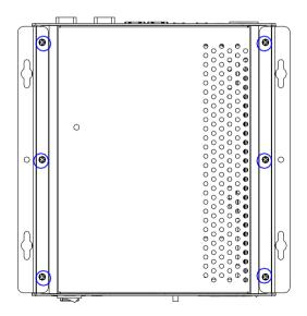
Step 6: Fasten the screws of front panel and rear panel
