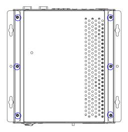
Step 11: Fasten the screws of front panel and rear panel
