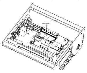
Step 8: Install the DIMM2 to the upper layer of the memory slot
