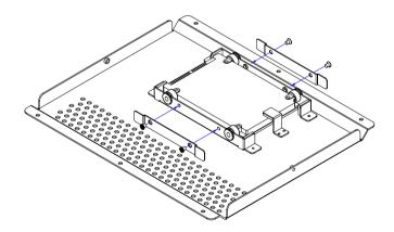
Step 4: Connect the HDD cable (SATA Type HDD)
