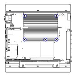
Step 4: Install the CPU module and fasten the screws
