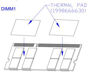
Step 5: Adhere the two thermal pads (1998666630) to the diode of the other side of memory DIMM1
