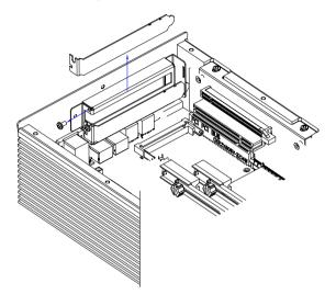
Step 4: Insert the PCI card into the PCI slot and reattach the screw.
