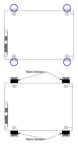
Step 2: Assembly the HDD chassis
