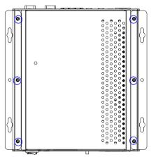
Step 8: Fasten the screws of front panel and rear panel
