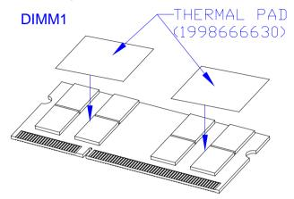
Step 6: Adhere the two thermal pads (1998666630) to the diode of facade of memory DIMM 2
