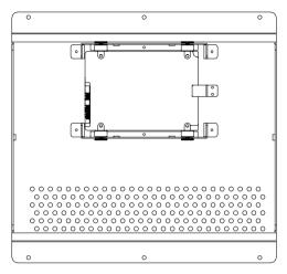
Step 3: Assembly the damper bracket
