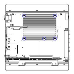
Step 4: Adhere the two thermal pads (1998666630) to the diode of facade of memory DIMM 1
