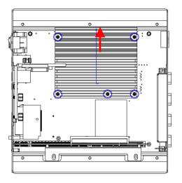
Step 10: Fasten the six screws on the back of the AEC-6940
