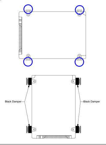
Step 2: Assembly the HDD chassis
