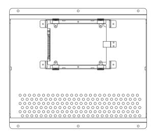
Step 3: Assembly the damper bracket
