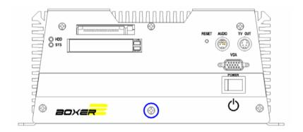
Step 2: Unfasten the screw on the front panel.
