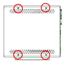
Step 2: Unfasten the four screws on the HDD cover.
