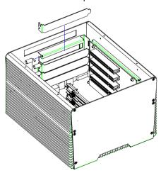
Step 3: Insert the PCI card into the PCI slot and reattach the screw.
