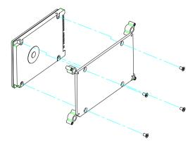
Step 4: Fasten the four screws to lock the HDD
