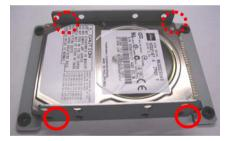
Step 3: Fasten the second HDD module to the bracket with screws.
