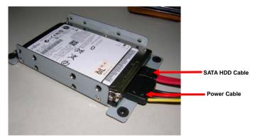
Step 4: Insert the HDD cable into the slot on the HDD module.
