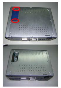
Step 2: Insert the other side of HDD cable and power cable into the slots on the bottom of the chassis.
