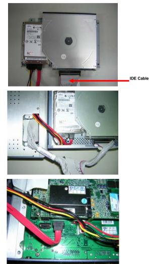
Step 6: Place the CD-ROM and HDD kit into the suitable plate and then reverse it. Screw the CD-ROM and HDD kit to the plate.
