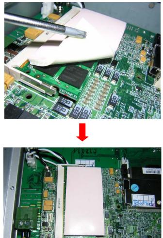
Step 2: Cover the chips with a thermal pad
