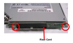
Step 4: Fasten the 2.5" HDD module to the disk bracket with screws.
