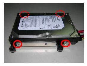
Step 4: Fasten the HDD module to the bracket with screws.
