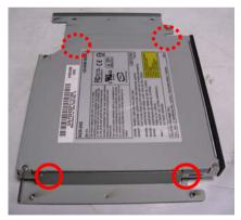
Step 3: Fasten the Riser Card and the CD-ROM with screws.
