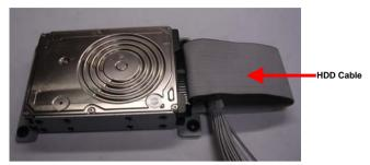
Step 5: Place the HDD kit into the HDD kit housing and then screw the HDD kit onto the HDD kit housing.
