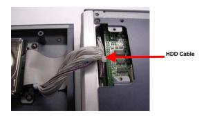
Step 3: Combine the chassis with the HDD kit housing and then lock with screws.
