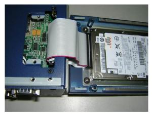
**Step 4:** Combine the HDD kit house with the chassis and push as the illustration shown below.
