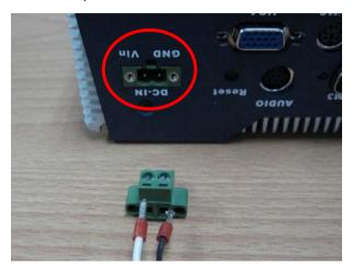
Step 4: Screw the power cable into the chassis.
