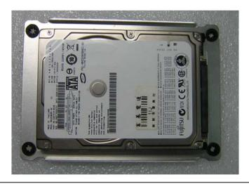
**Step 3:** Stack the HDD and bracket. Fasten HDD and bracket with the screws.
