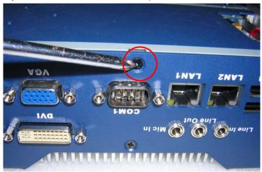
**Step 3:** Unfasten the four screws on the bottom case of AEC-6831
