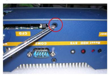
Step 2: Loose the screw on the rear panel of AEC-6831
