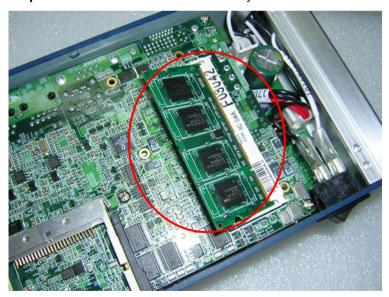
**Step 5:** Press the SDRAM and make sure that it has been inserted properly
