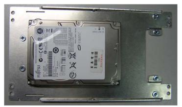
**Step 2:** Fasten the four screws with the bottom cover of AEC-6821
