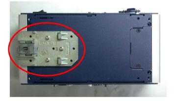
Step 2: Press the DIN Rail on the DIN Rail kit to fix it.
