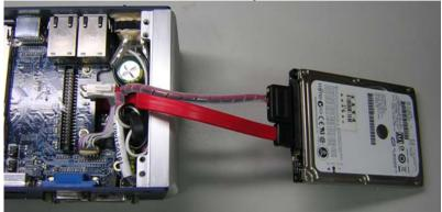
**Step 6:** Insert the Cable to the bottom of the chassis as the illustration below.
