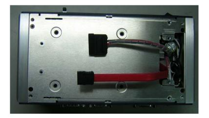
**Step 7:** Connect the IDE/ SATA and power cables to the Hard Disk Drive kit
