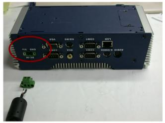
Step 4: Screw the power cable into the chassis.
