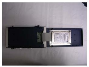
**Step 3:** Combine the HDD kit house with the chassis and push as the illustration shown below.
