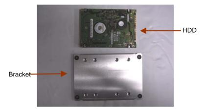
**Step 1:** Stack the HDD and bracket. Fasten HDD and bracket with the screws.
