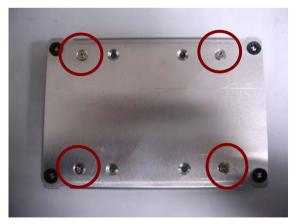
Step 2: Fasten the HDD module into the HDD kit house.
