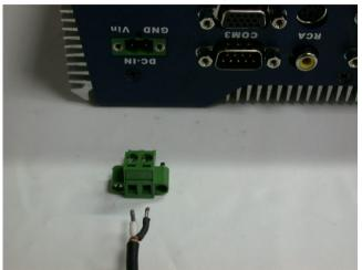
Step2: Fix the connector to the cable with the screws.
