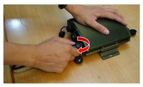
Step 3: Connect the VGA cable connector to the monitor and turn
