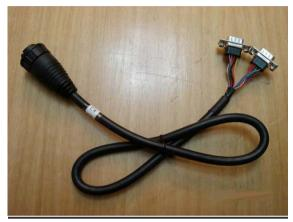
Step 1: Remove the C4 cable from the accessory kit
