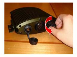
**Note 2:** Please pay attention on the key of the cable connector when you connect the cable connector to AEC-6710. The notch of the cable connector should be in the upper position. Another way to connect properly is to identify the characters of "**LTW**" on the cable connectors. (See Photo below) The "LTW" should be on the top of the connector.
