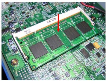
Step 2: Adhere the heat spreading pad to the RAM
