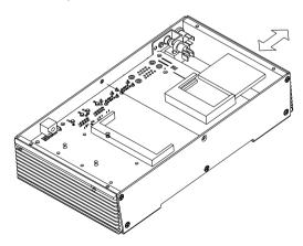
Step 3: Fasten the six screws to close the case of AEC-6620, and you have finished the CompactFlash<sup>TM</sup> installation
