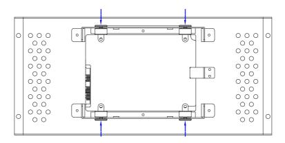
Step 5: Assemble the damper bracket
