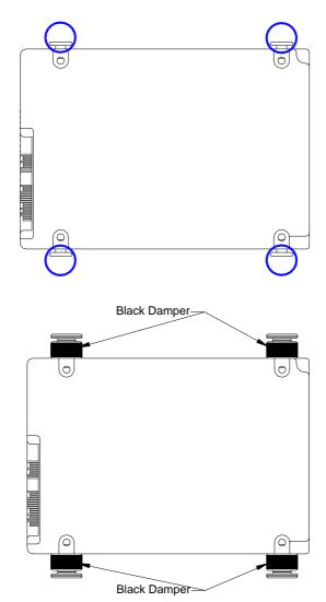
Step 4: Assemble the HDD chassis
