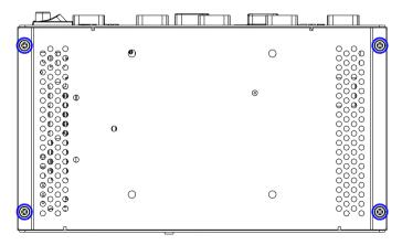
Step 3: Fasten the four HDD screws and cover with the four black damper
