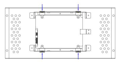
Step 5: Assembly the damper bracket
