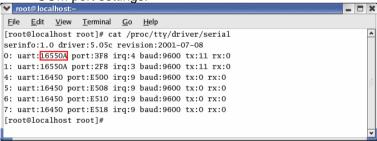
As the screen showing, use 16550A to be UART prefix is the system COM ports, and we can see this system with 2 COM ports, leave it as ttyS0, ttyS1. Make Ispci -v command to find OXmPCI952 IRQ and I/O address
