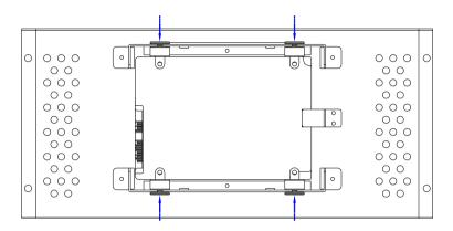
Step 5: Assembly the damper bracket
