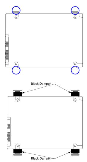
Step 4: Assembly the HDD chassis
