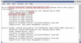
As the screen showing, we can find "Serial controller: Oxford Semiconductor Ltd:" this alphabetic string and then we will see the next line with IRQ number and the next with I/O address
