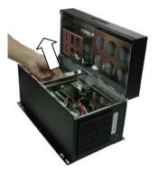
• Unscrew the hold-down bar and remove it.
