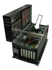
• Screw the hold-down bar to the same location from where it was removed in the first step.
