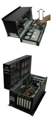
• Unscrew the mounting bracket from the chassis.
