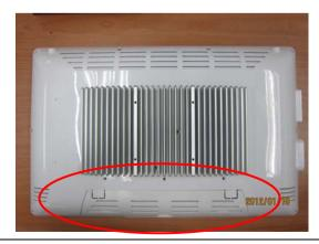
**Note 1:** You may turn on the power by cutting and destroying the protective cover as it shows below.
