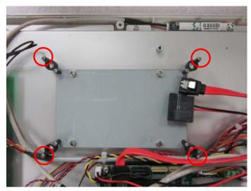
Step 4: Get the HDD and HDD Bracket ready
