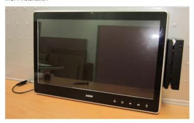
Step 1: Fasten the two screws (2-SELF TAPPING SCREWS) to fix the MSR Bracket with the ACP-5217
