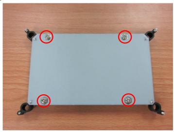
Step 6: Connect the SATA and power cables to the HDD and fasten the four screws to fix the HDD Bracket
