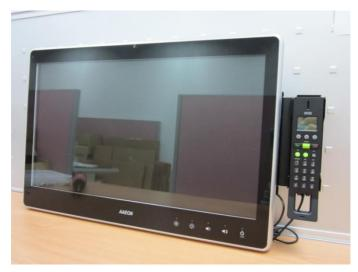
Step 1: Fasten the two screws(2-SELF TAPPING SCREWS) to fix the Skype Bracket with the ACP-5210
