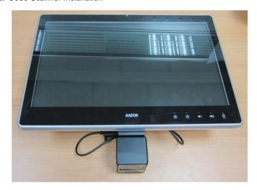
Step 1: Fasten the three screws to fix the Bar Code Scanner with the backet
