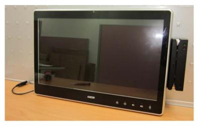
Step 1: Fasten the two screws (2-SELF TAPPING SCREWS) to fix the MSR Bracket with the ACP-5187
