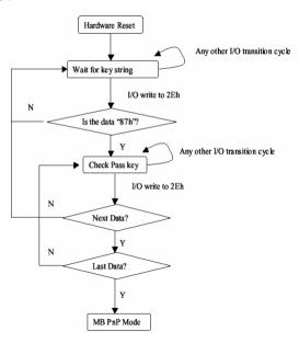
There are three steps to complete the configuration setup: (1) Enter the MB PnP Mode; (2) Modify the data of configuration registers; (3) Exit the MB PnP Mode. Undesired result may occur if the MB PnP Mode is not exited normally.
