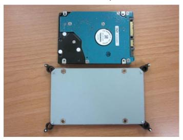
Step 5: Fasten the four screws to fix HDD Bracket and HDD
