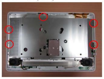
Step 3: Remove HDD Bracket (4 screws)
