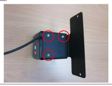
Step 2: Fasten the two screws (2-SELF TAPPING SCREWS) to fix the Bar Code Scanner with the ACP-5187
