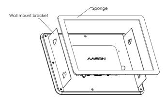
**<u>Step 2</u>**: Remove the six screws (three on each side) at the back and place the wallmount brackets onto the display. Secure the brackets with the original six screws.
